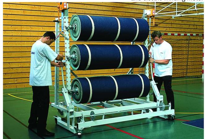
hanging the rolls into the rack with the off- and onrolling device
