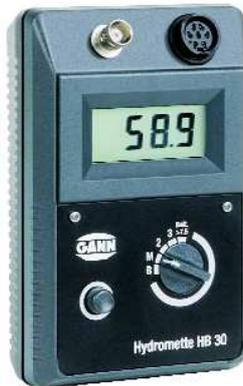
Professional set in plastic case for wood and other construction materials. Also delivered with Active-Electrode B50
