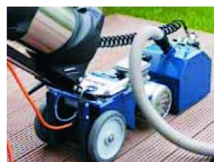
connection of an external dust extractor
