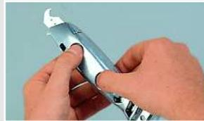
Unlocking of blade chamber.
