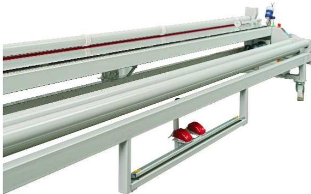
2. The continuous insertion pressure drum is operated with the foot pedal on the front side of the machine and can be raised or lowered with a hoist cylinder.
