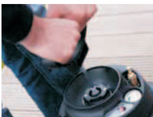
Hand operated pumping to produce pressure in the oil tank
