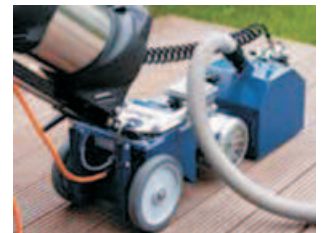
Connection of an external dust extractor
