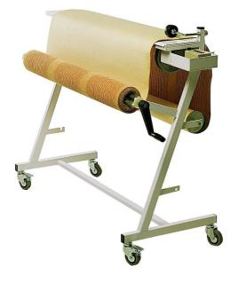
The FMS 1100 measuring and cutting device is suitable for roll widths up to 110 cm, while the FMS 1500 is suitable for widths up to 150 cm.
