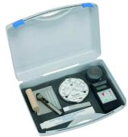
complete with: floor-air-thermometer, moisture indicator Caisson V1-D1, thermo-hygrometer TH100, subfloor hardness meter, screed level measuring wedge, folding rule
