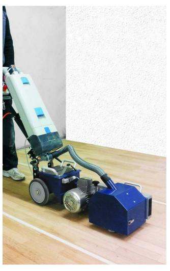
direct connection of the suction hose to the dust extractor GK40
