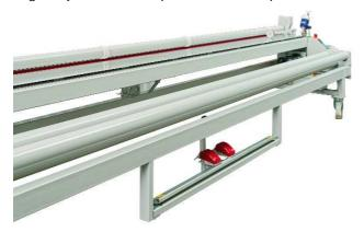
The continuous insertion pressure drum is operated with the foot pedal on the front side of the machine and can be raised or lowered with a hoist cylinder.
