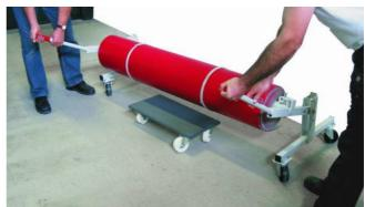
Roll lifter hand-operated for 200 cm (6'6"), 400 cm (13 ft) and 500 cm (16'4") material width
