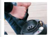
Hand operated pumping to produce pressure in the oil tank
