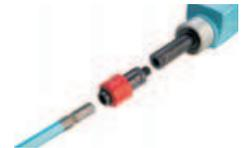
Combi-adapter for upgrading handheld stirring machines with HEXAFIX® to M14 thread. Screw the combi-adapter onto the 5/8 thread of the handheld stirring machine instead of the Hexafix®-coupling.
