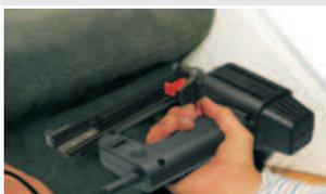
Using the MET 4000 for fixing stretched carpets
