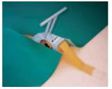
Off- Roller Type DF for application of double sided tape
