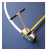
Marking Head with 50 mm Marking Tape
