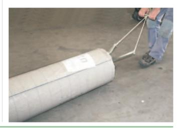
Roll Lifter hand-operated for 200 cm (6'6"), 400 cm (13 ft) and 500 cm (16'4") material width
