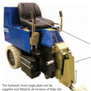
Blade angles can be adjusted quickly and precisely by the operator without having to get off the machine. This saves time, especially on building sites with different floor removal requirements.
