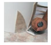
Edge-cutting tool for textile, PVC and CV Coverings
