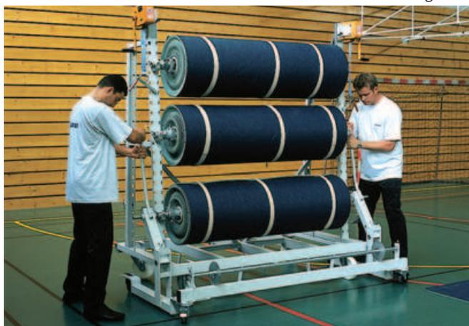
hanging the rolls into the rack with the Transport and Unroll Trolley
