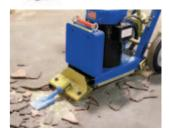
Adjustment of cutting angle
