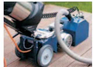
Connection of an external dust extractor
