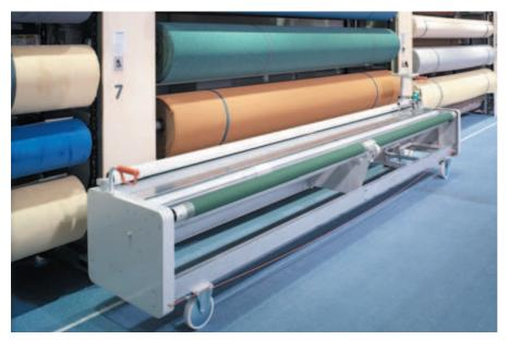
With cutting tables, rolls can be easily unrolled from paternosters, measured, cut and packed.
