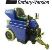
The batteries should be replaced after approximately 400 charging cycles.
