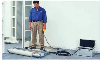
Near walls only a strip of approx. 10 cm (4") has to be removed manually. The rest of the job is done by the ELEPHANT almost automatically
